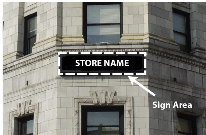
Figure B: Illustration of computing the sign area for wall signs with a background panel or cabinet.
